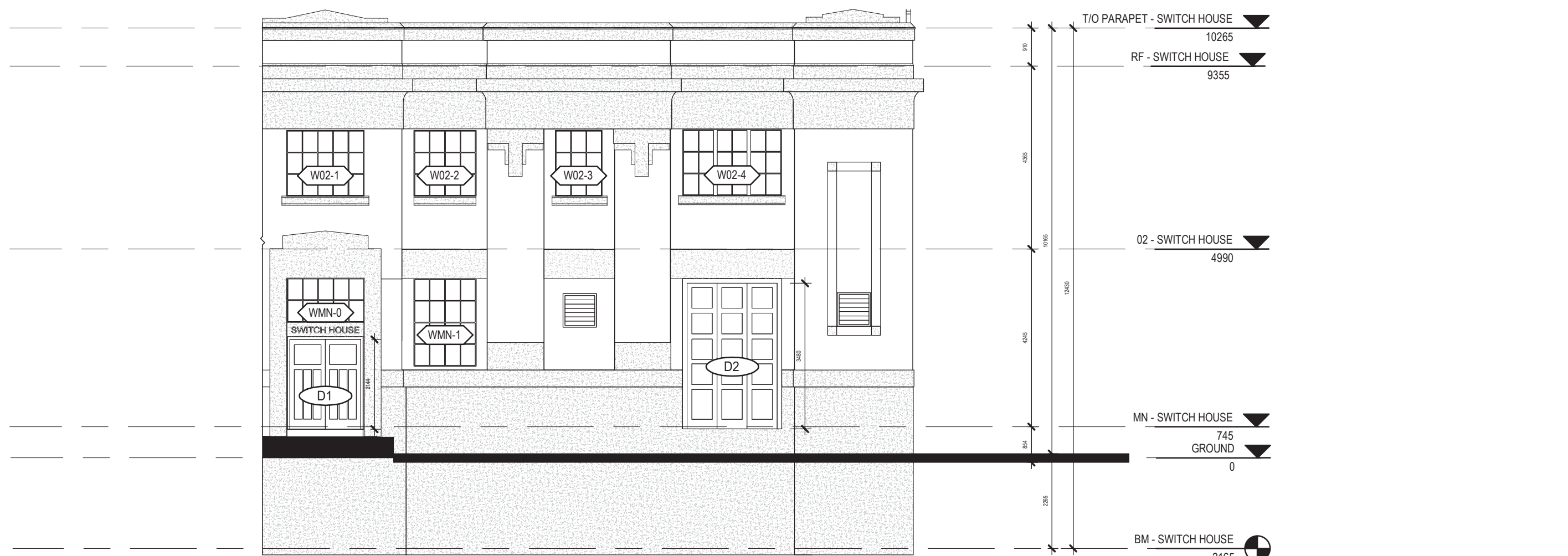
1 SOUTH ELEVATION SWITCH HOUSE 1 : 100
