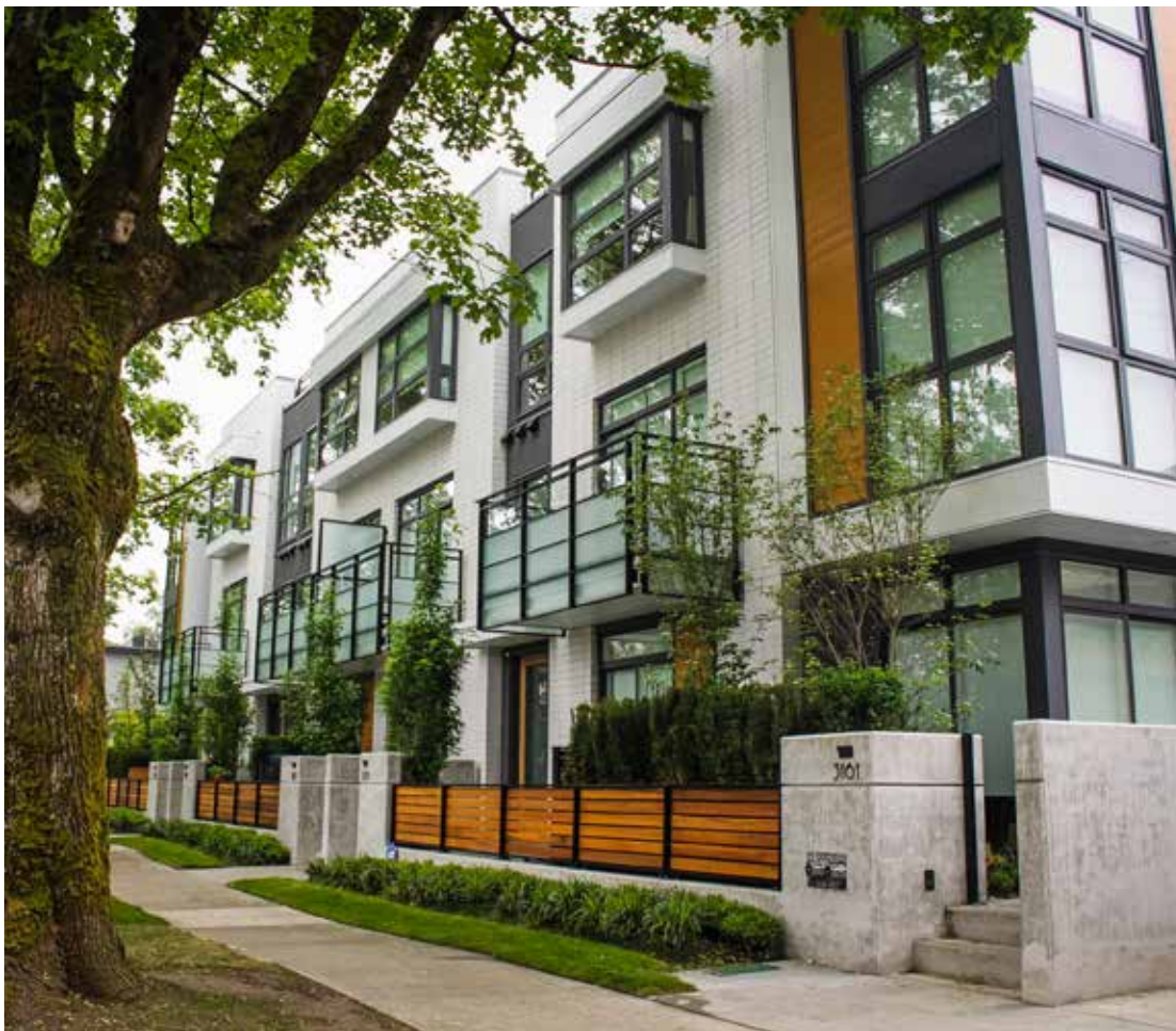
Ground floor entrances with forecourts separated from the street by low fences and grade separation to enhance privacy [2].
