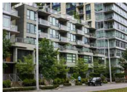
A building that addresses the street with a varied and engaging visual experience, incorporating recesses, projections, setbacks, building segmentation and changes in window type [2].
