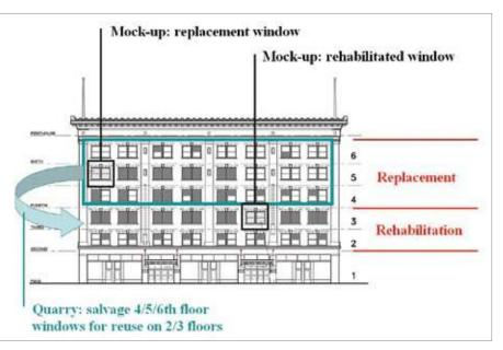
While rehabilitating the Lougheed Building in Calgary, the windows in the best condition were repaired and consolidated on the lower levels where they were most visible from the street. New windows based on the existing were specially constructed for the upper levels. The location and reuse of the windows was carefully and clearly documented both for construction purposes and for future reference.
