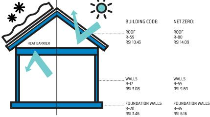
Note that a Heat Recovery Ventilator (HRV)—see **Ventilation Information** chapter was assumed to be in use for both the building code and net zero R-value examples above; without an HRV, the R-values will typically increase.
