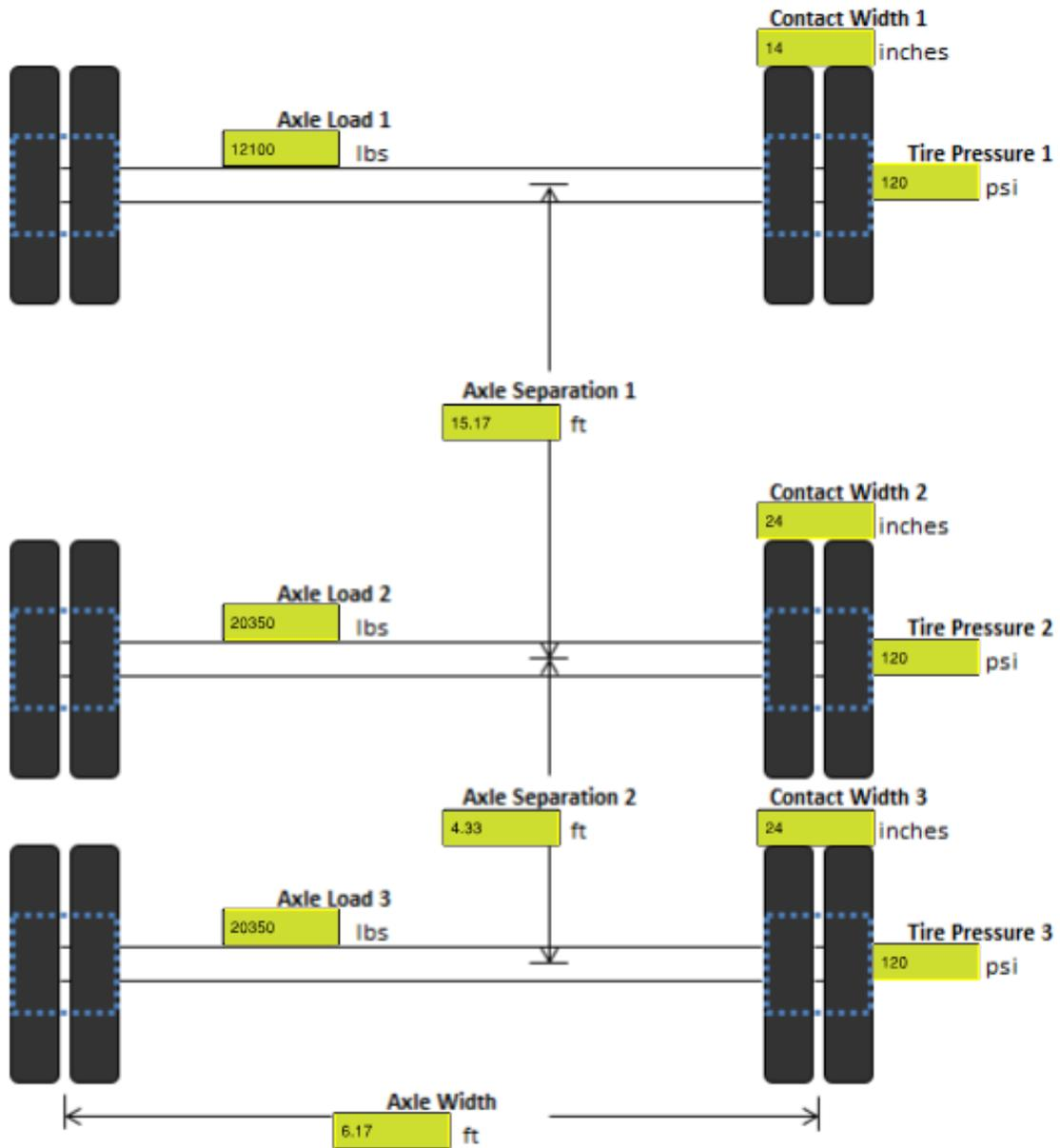
Figure 5-1E.1: Tandem Gravel Truck (Loaded)
