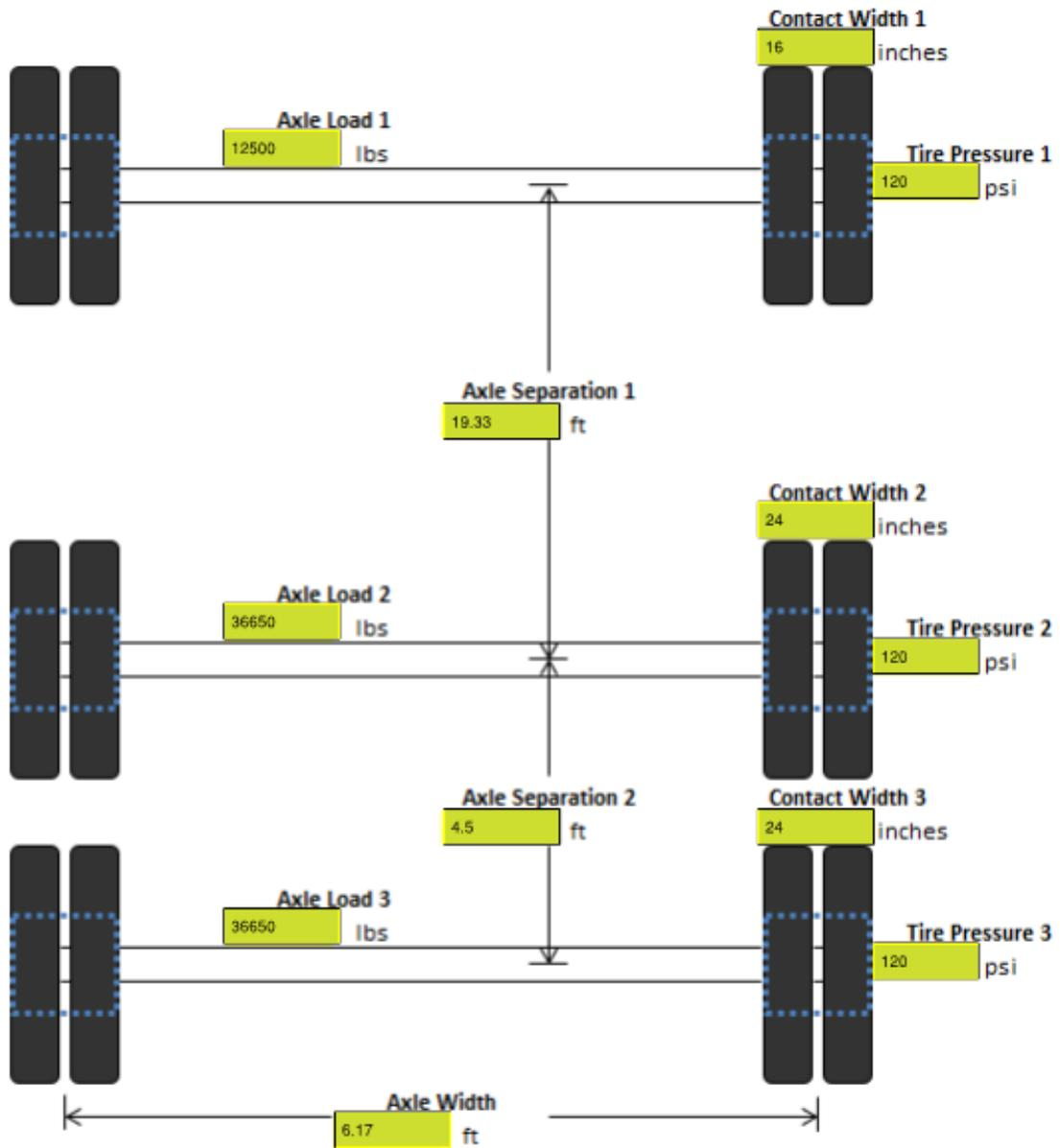
Figure 5-1E.2: Tandem Picker Truck (Loaded)
