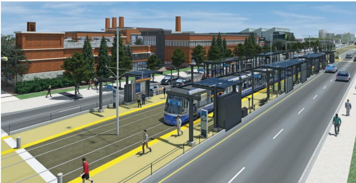
Low-floor LRT vehicles were first introduced in the late 1980s and have since evolved to become the industry standard for new LRT systems in Europe and North America. Most of the mechanical equipment on a low-floor LRT vehicle is located on the roof, which means the train doors open at street level for step-free boarding onto the vehicle.
