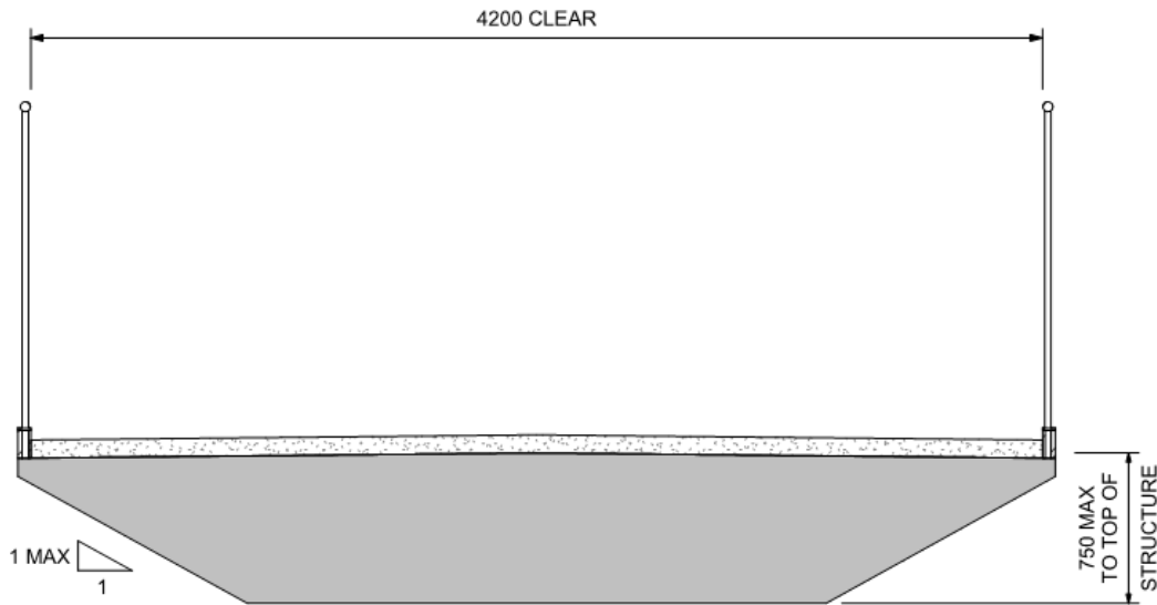
Figure 2-11.7.2: Kâhasinîskâk Bridge Superstructure Section (dimensions in mm)
