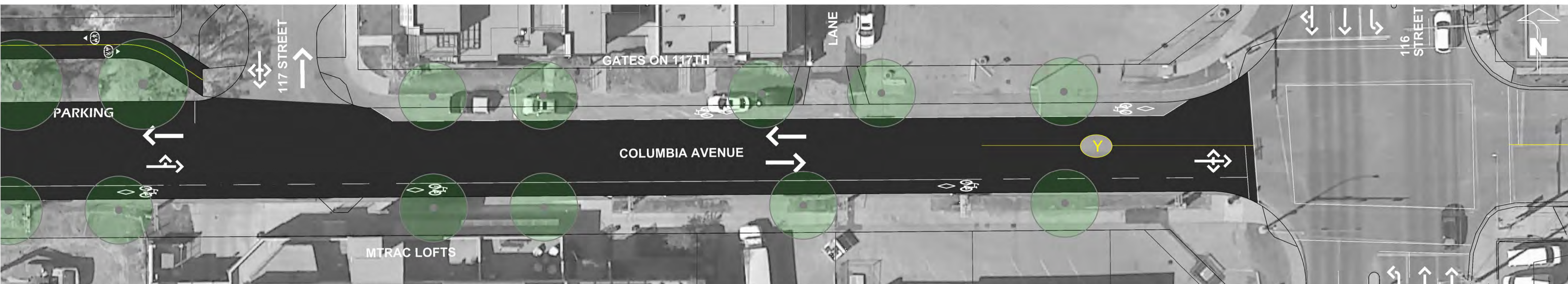
MAINTAIN EXISTING - ONE-WAY UNPROTECTED BIKE LANES - TWO-WAY VEHICLE TRAFFIC WITH PARKING WEST OF 117 STREET
