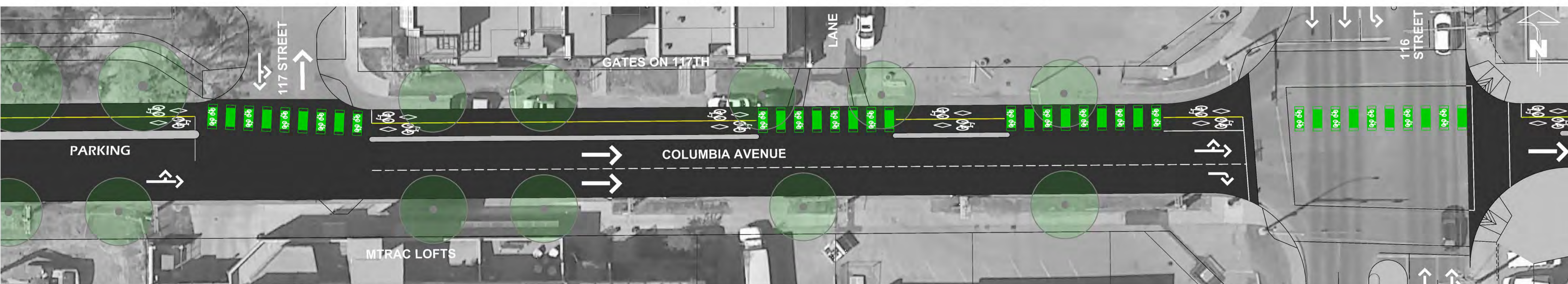
OPTION B - TWO-WAY PROTECTED BIKE LANE - ONE-WAY VEHICLE LANE WITH PARKING LANE WEST OF 117 STREET
