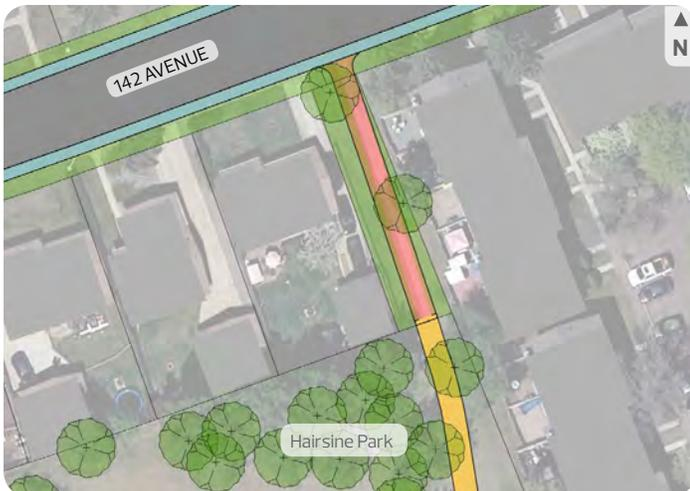
Figure 32. Enhanced breezeway location B - Plan
