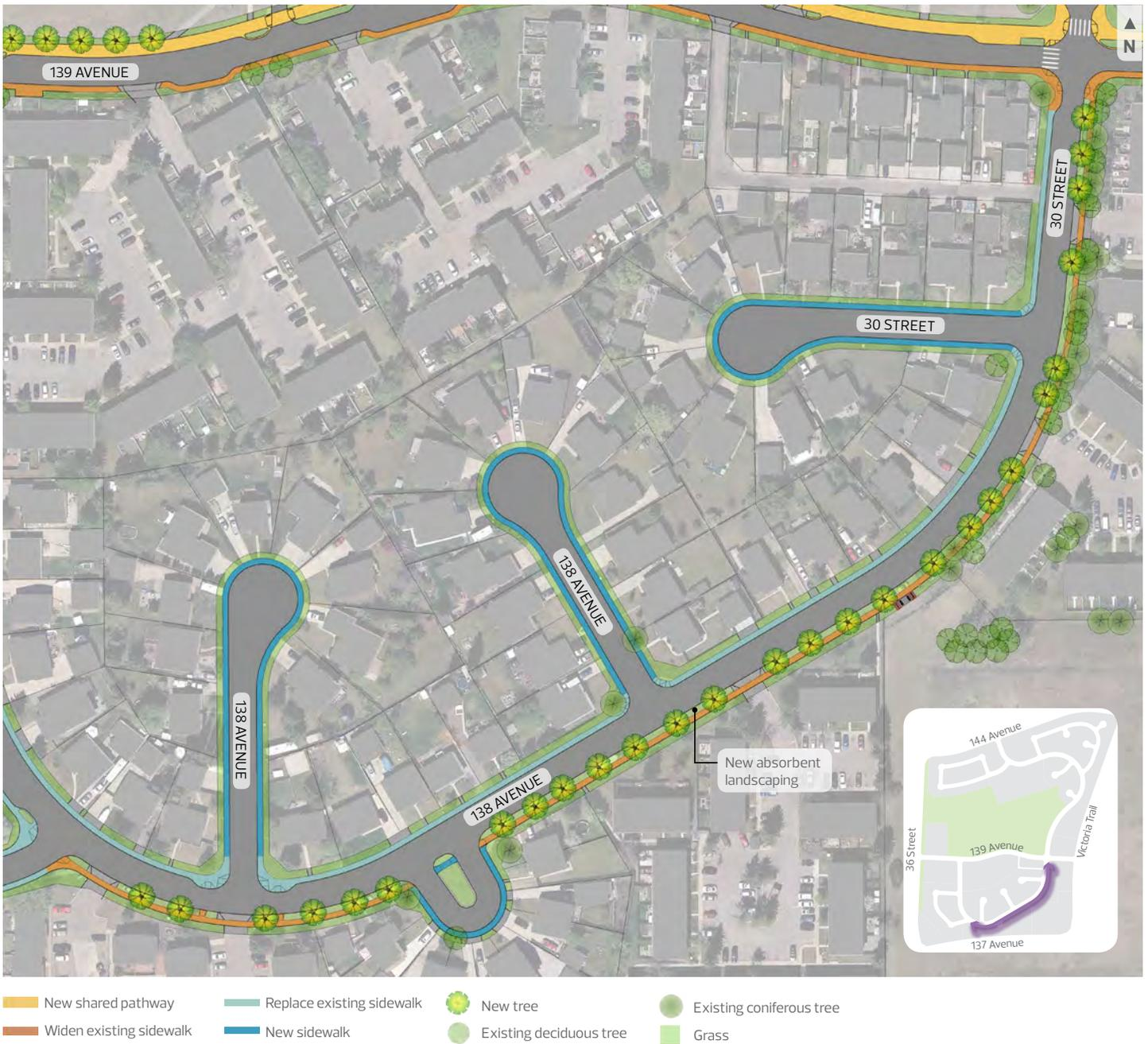
Figure 20. New boulevard along the local loop road of 142 Avenue/30 Street/138 Avenue - Plan: South portion
