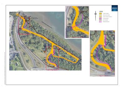
The first trail connection (labelled as Staircase Connection Walkway) will connect the existing stairway from Groat Road, including a pedestrian crossing across the park road, and to the river valley trail system. The trail will be constructed out of gravel.
