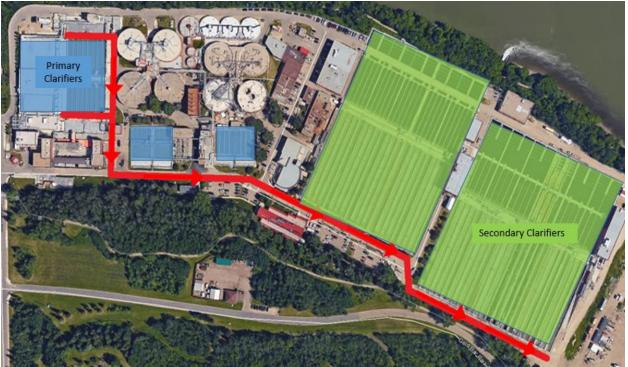
Figure 2.0-1 Primary Effluent Channel Path
