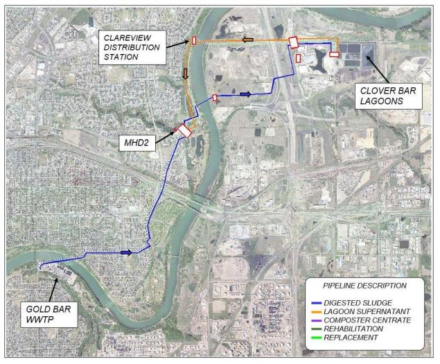
Figure 2.1-2 Sludge and Supernatant Pipeline Typical Flow Paths
