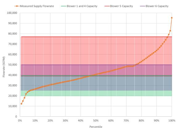
Figure 2.0-1 Percentile Distribution of Measured Flowrates and Blower Capacities
