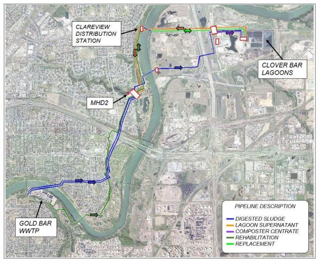
Figure 2.1-1 Sludge and Supernatant Pipeline Overview
