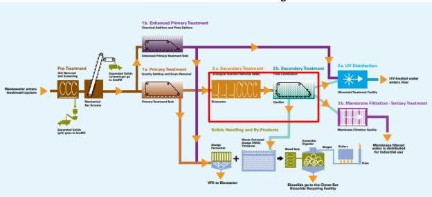
Figure 1.0-1 Gold Bar WWTP Process Flow Diagram
