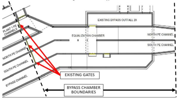
Figure 2.0-3 Current Configuration of the Bypass Chamber
