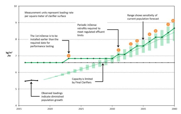
24. Providing performance is satisfactory, three inDENSE<sup>™</sup> systems will be added in the 2030-2034 PBR and four more will be installed in the 2035-2039 PBR, based on the capacity requirement. If inDENSE<sup>™</sup> performance does not meet expectation, detailed design of the first MBR conversion will be initiated by 2024 with construction completing by 2028.
