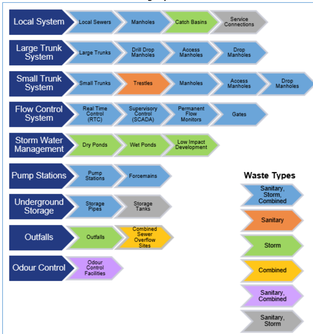
Figure 3.1.1-1 EWSI’s Drainage System Overview
