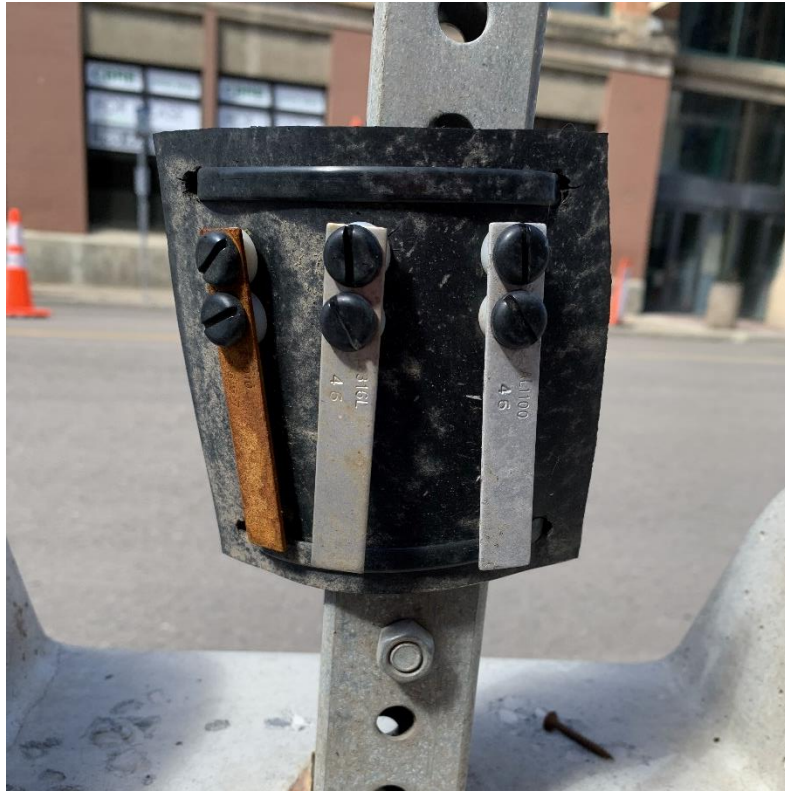
Figure 10 - Corroded Coupons Installed on Bicycle Lanes (Left to Right: Carbon Steel, Stainless Steel and Aluminum)
