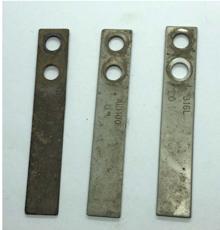
Figure 8 - Corroded Bus Coupons Installed on Spruce Grove Bus (Left to Right: Carbon Steel, Aluminum And Stainless Steel)
