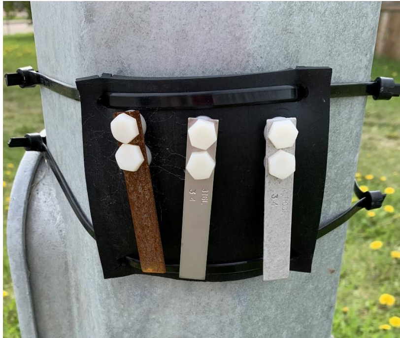
Figure 9 - Corroded Field Coupons Installed On 178 Street (Left to Right: Carbon Steel, Stainless Steel and Aluminum)
