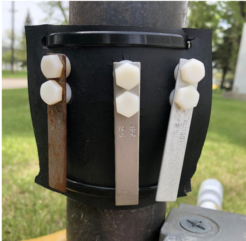
Figure 11 – Corroded Environmental Control Field Coupons Installed Near Corrpro Office (Left to Right: Carbon Steel, Stainless Steel and Aluminum)
