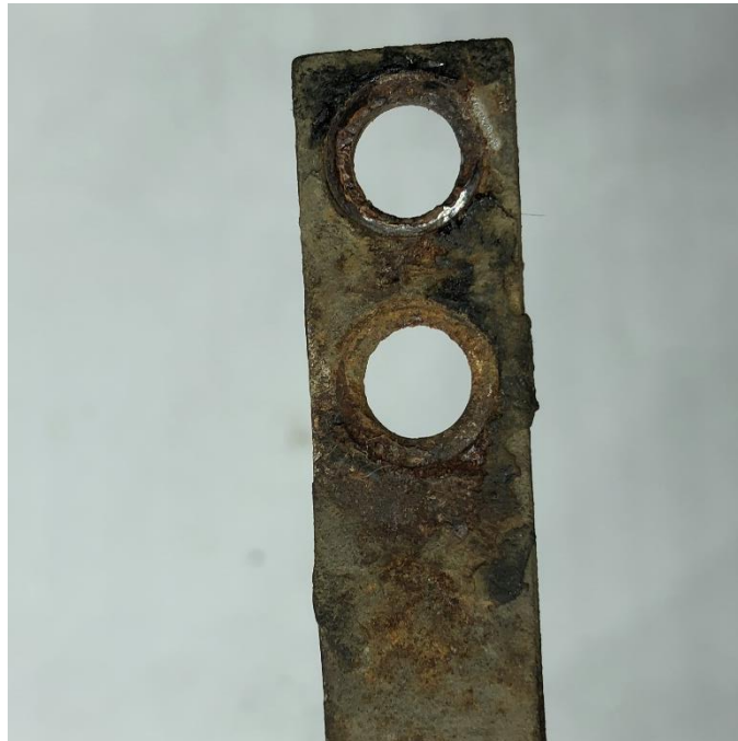
Figure 12 - Crevice corrosion on carbon steel coupon
