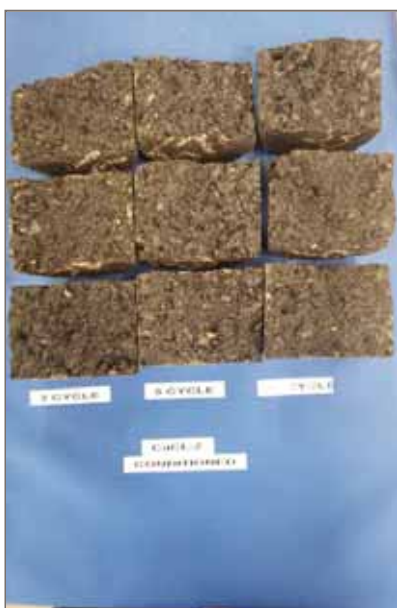
Photo 3: TSR Test Test results of conditioned samples for 3, 5, and 10-Cycle exposure in NaCl/CaCl 2 -2 solution
