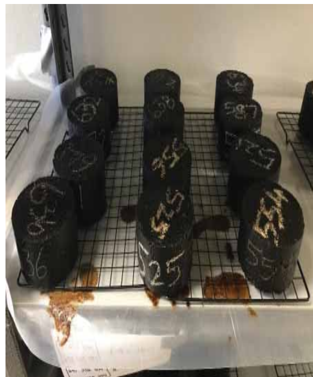
Photographs 5 and 6: Drying Apparatus Used Between Exposure Cycles
