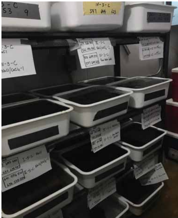
Photographs 3 and 4: Example of Submerged Specimens in Chemical Solution
