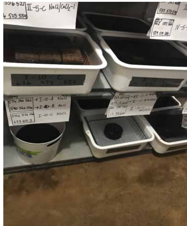
Photographs 3 and 4: Example of Submerged Specimens in Chemical Solution
