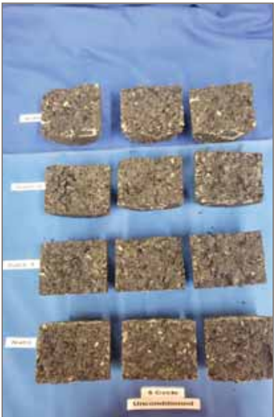
Photo 10: TSR Test Test results of unconditioned samples in NaCl, NaCl/CaCl 2 -1, NaCl/CaCl 2 -2, and water solutions for 5-Cycle exposure
