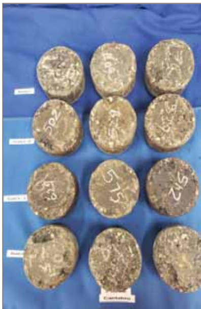
Photo 5: Cantabro Test Test results/samples in NaCl, NaCl/CaCl 2 -1, NaCl/CaCl 2 -2, and water solutions for 3-cycle exposure
