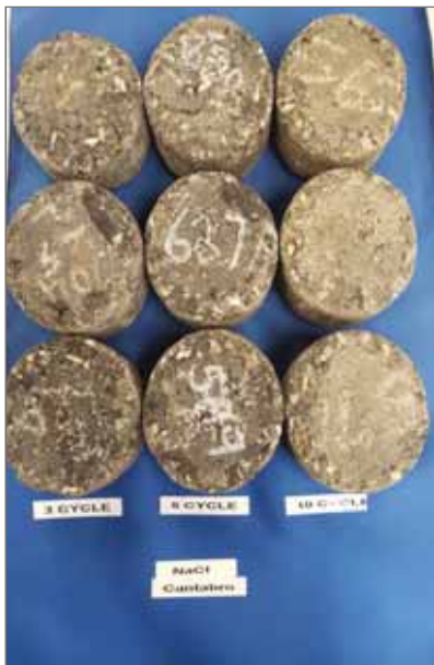
Photo 1: Cantabro Test Test results/samples for 3, 5, and 10 cycle exposure in NaCl solution
