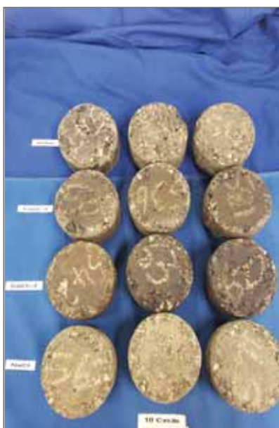
Photo 7: Cantabro Test Test results/samples in NaCl, NaCl/CaCl 2 -1, NaCl/CaCl 2 -2, and water solutions for 10-cycle exposure
