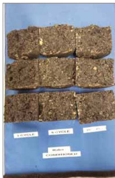
Photo 4: TSR Test Test results of conditioned samples for 3, 5, and 10-Cycle exposure in water solution
