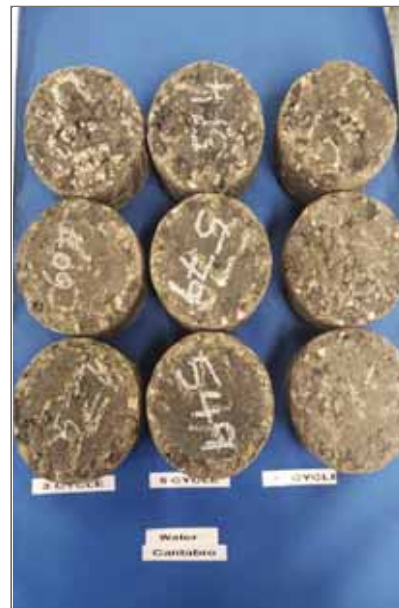
Photo 4: Cantabro Test Test results/samples for 3, 5, and 10 cycle exposure in water solution
