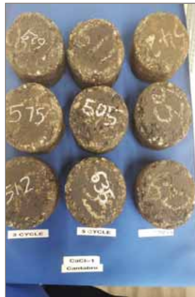
Photo 2: Cantabro Test Test results/samples for 3, 5, and 10 cycle exposure in NaCl/CaCl 2 -1 solution
