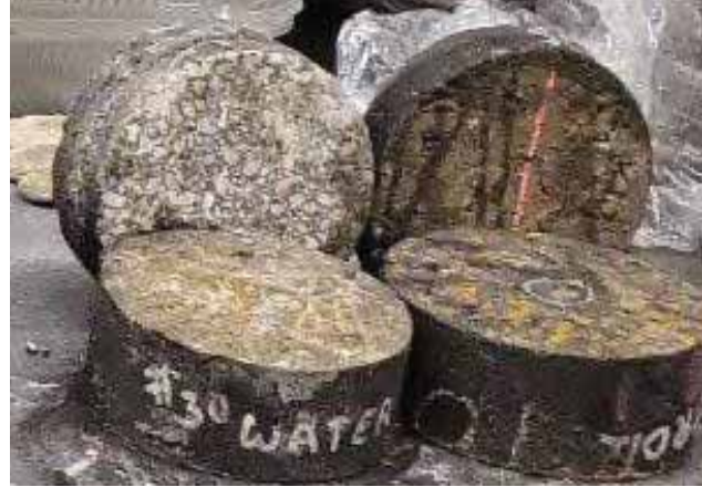
Figure 1: Specimens saw-cut to the height of 6 \pm 0.1 cm
