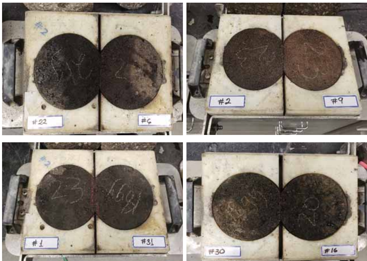
Figure 2: Specimens saw-cut along a secant line (ready for testing)
