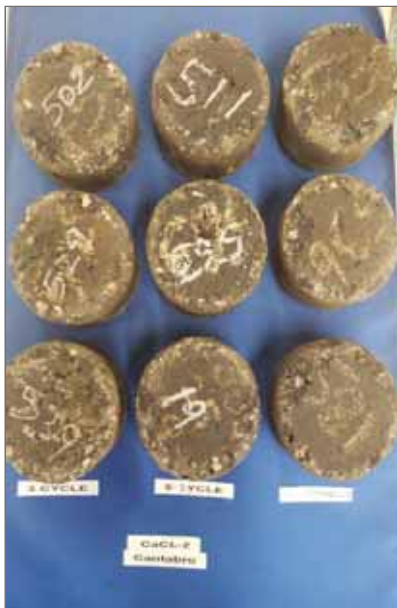
Photo 3: Cantabro Test Test results/samples for 3, 5, and 10 cycle exposure in NaCl/CaCl 2 -2 solution
