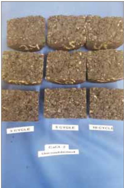
Photo 7: TSR Test Test results of unconditioned samples for 3, 5, and 10-Cycle exposure in NaCl/CaCl 2 -2 solution
