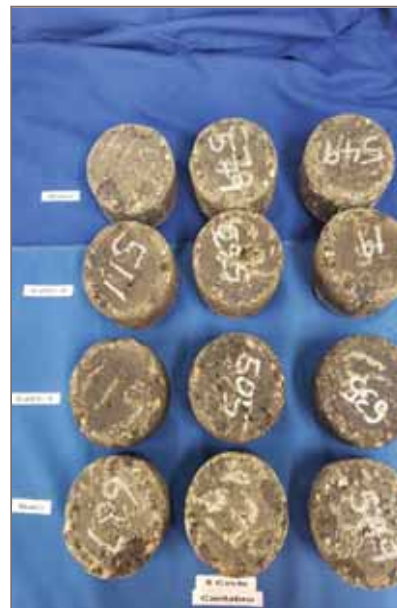
Photo 6: Cantabro Test Test results/samples in NaCl, NaCl/CaCl 2 -1, NaCl/CaCl 2 -2, and water solutions for 5-cycle exposure
