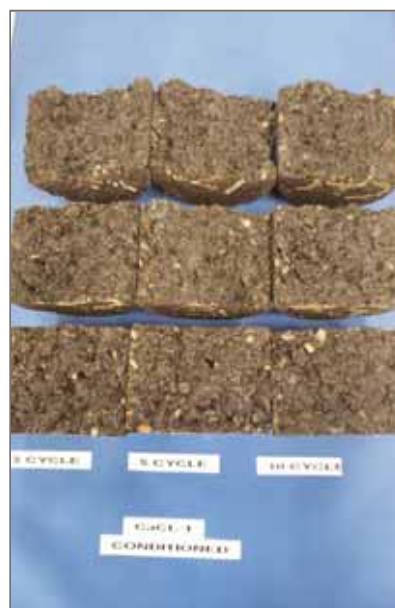
Photo 2: TSR Test Test results of conditioned samples for 3, 5, and 10-Cycle exposure in NaCl/CaCl 2 -1 solution
