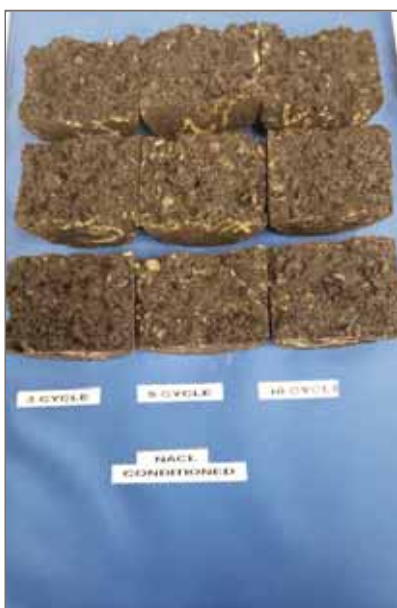
Photo 1: TSR Test Test results of conditioned samples for 3, 5, and 10-Cycle exposure in NaCl solution
