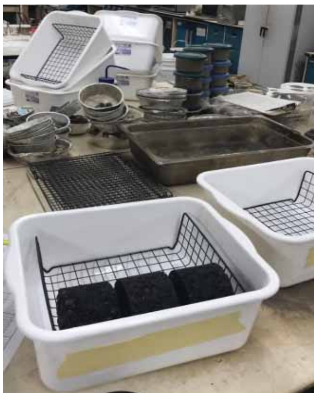
Photographs 1 and 2: General Configuration of the Chemical Exposure Apparatus
