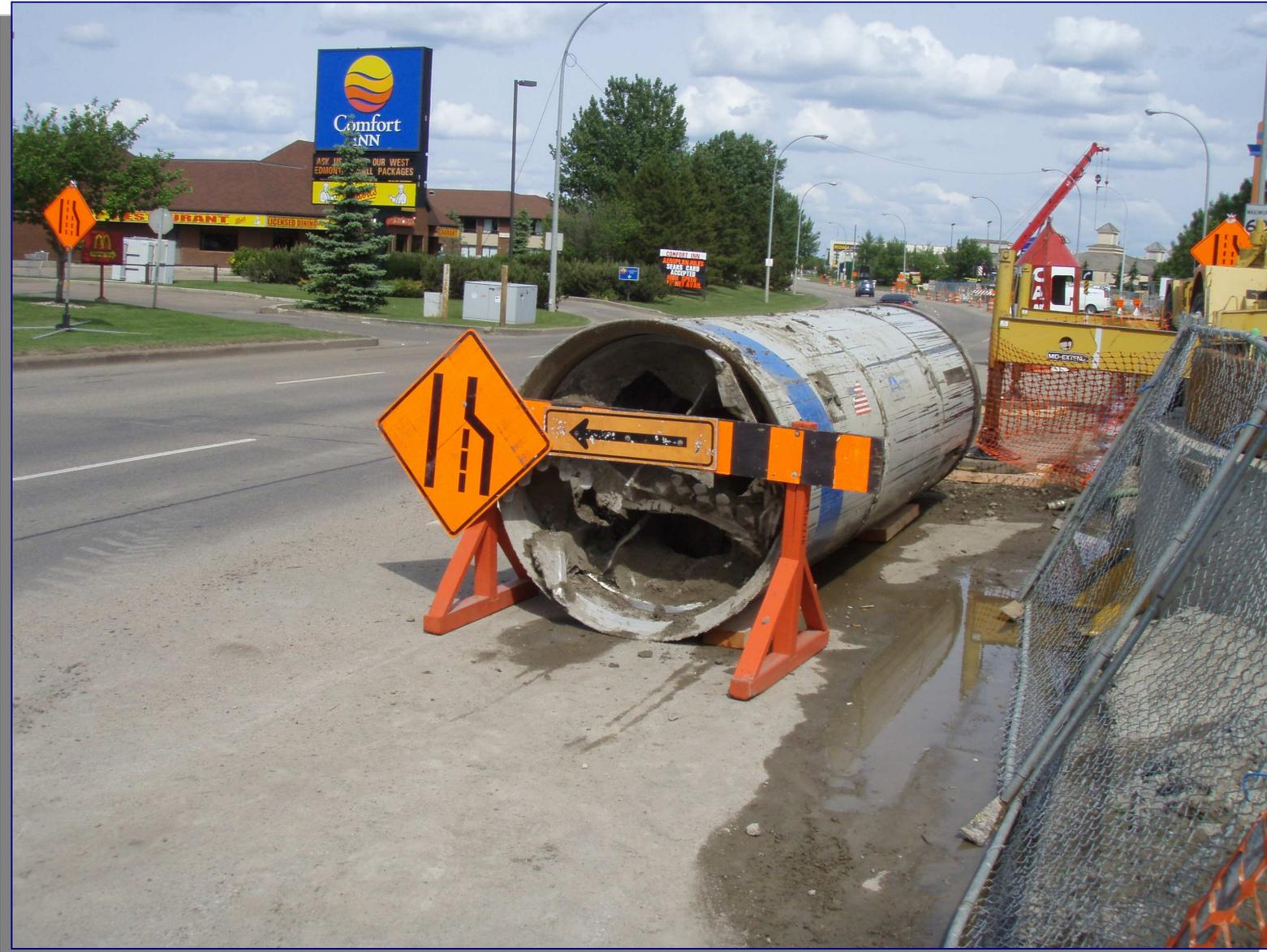
Figure 1a. WESS Stage W1: Micro Tunnel Machine head after the completion of run
