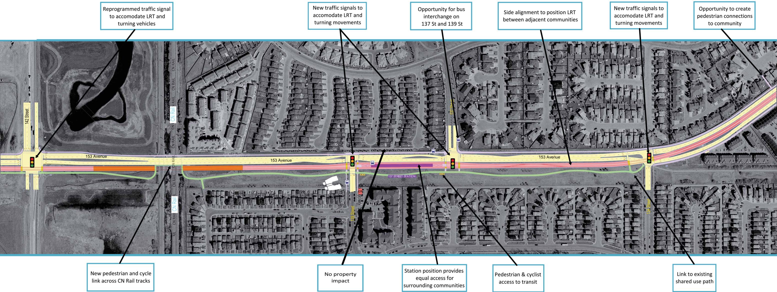
Reprogrammed traffic signal to accommodate LRT and turning vehicles
