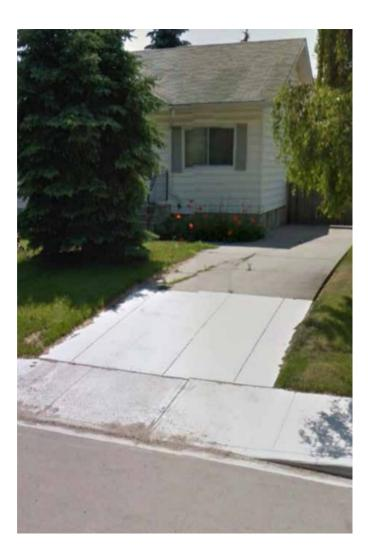
A portion of private walkway and driveway may need to be removed in order to tie into the new sidewalk elevation. The amount removed will depend on the new sidewalk elevation. The portion of private walkway and driveway that was removed will be replaced with the material that was originally removed
