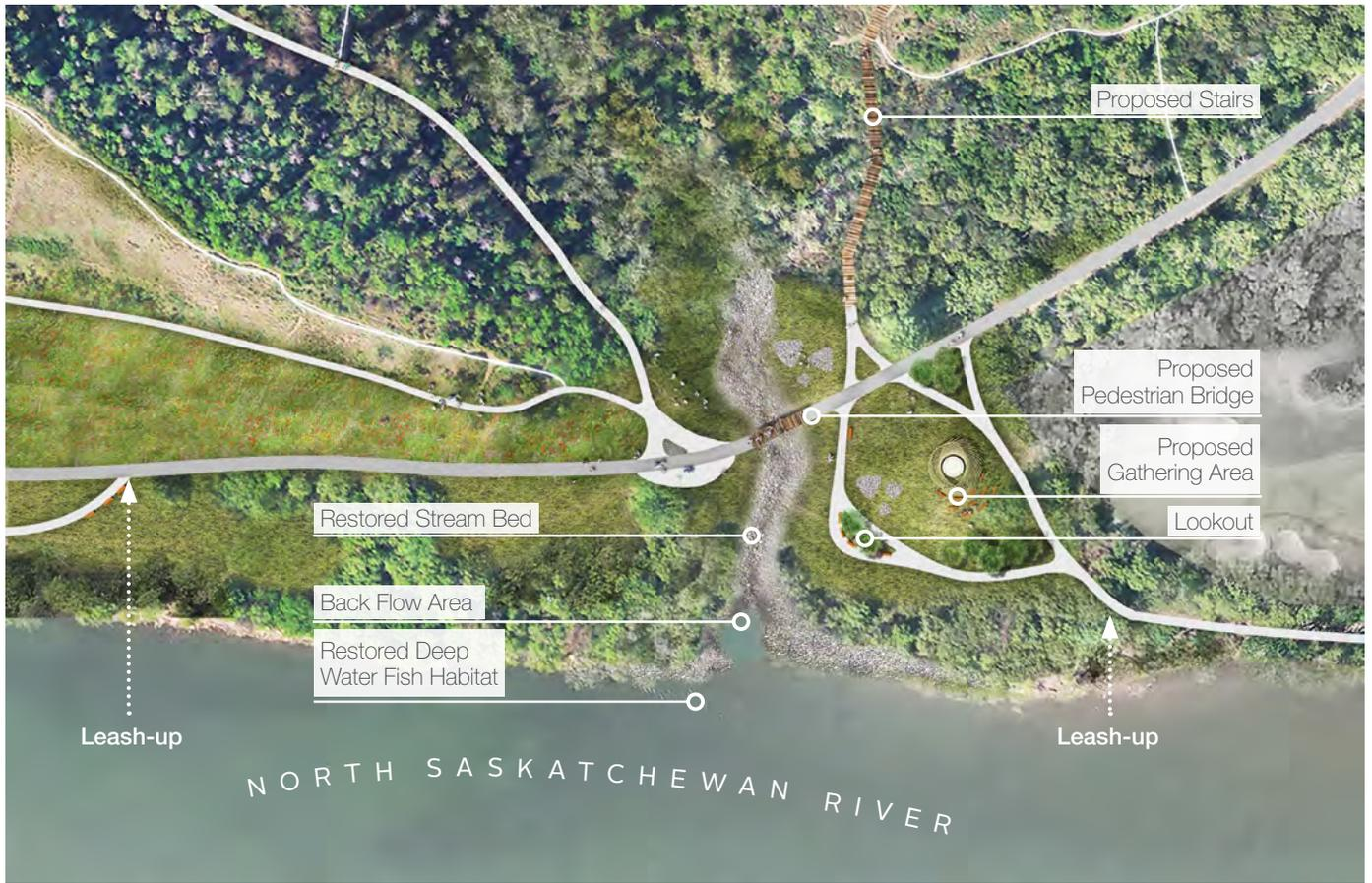
Figure 45. Rat Creek Restoration - Plan View
