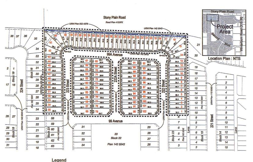
Construct a 2.4 m noise attenuation fence
