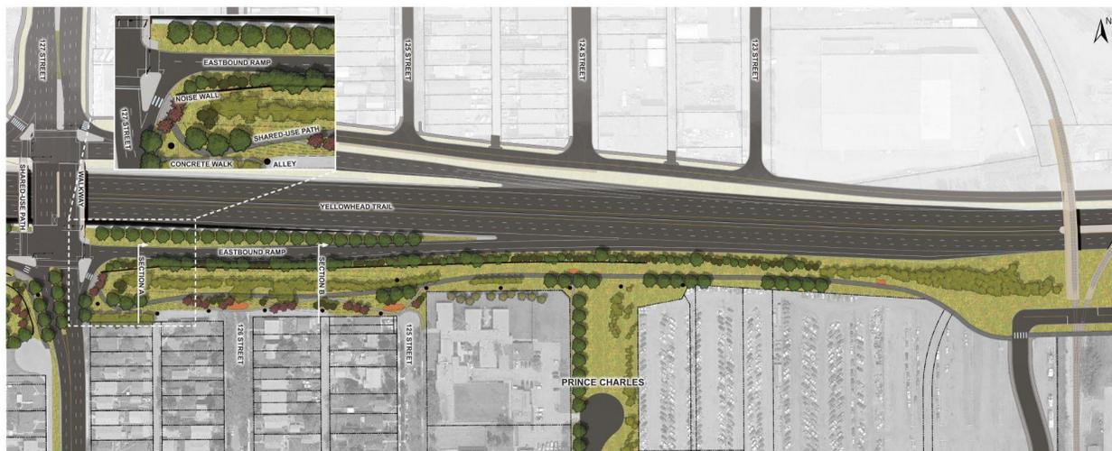
Option 1 provides a straight shared-use path on the top of the existing berm adjacent to the noise wall along Yellowhead Trail.
