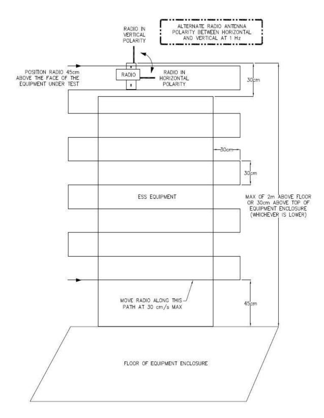
Figure 1: RSQT Testing Path
