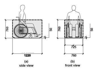
Figure 2: Wheelchair Movement Requirements
