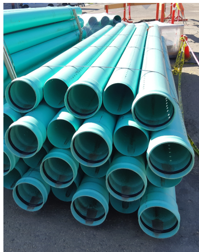
Photo 6: Perforated PVC Piping
