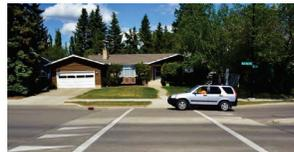
A crosswalk which is constructed higher than the roadway surface.
