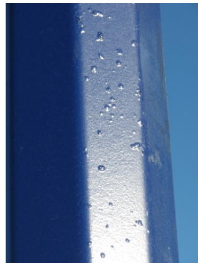
Figure 2: Bubbles in powder coating layer
