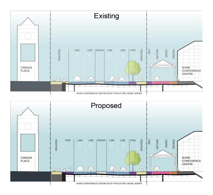
The proposed new cross section east of 97 Street provides barrier free 3 metre sidewalks along with a new furnishing zone on the north side of the avenue for an extended pedestrian gathering space plaza in front of Canada Place. While roadway widths have been reduced, the roadway lane structure remains the same with two travel lanes in each direction and a centre median.
