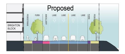
East of 96 Street the proposed new cross section includes wider, barrier free 3 metre sidewalks on each side of the avenue, along with a furnishing zone and new ancillary zone or flex space, which can be used for parking or pedestrian space (food trucks, patios, event space).
